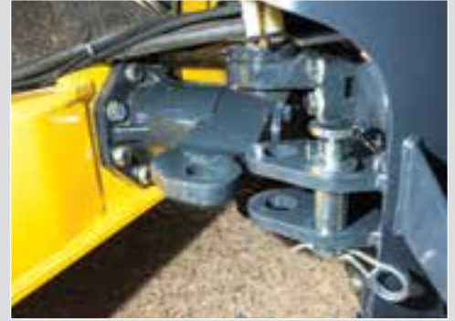
Bolt-on centerjoint is maintenance-free.
