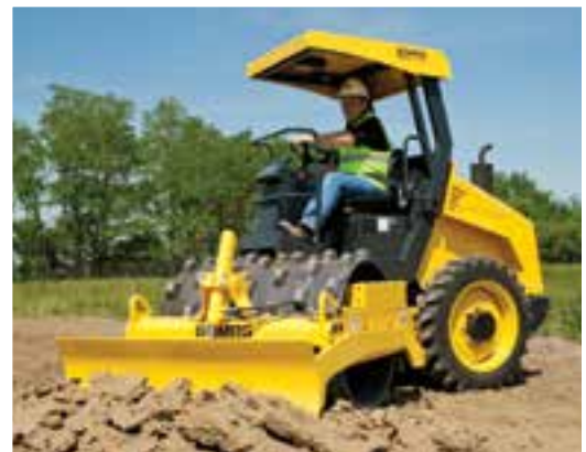
BW124PDH-40 padfoot roller with optional leveling blade.
