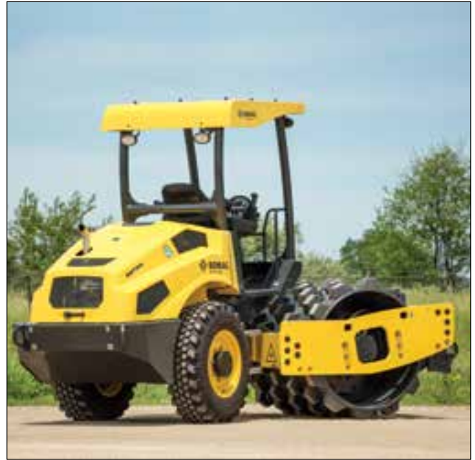
Operator's cockpit features dual entry accessibility.
