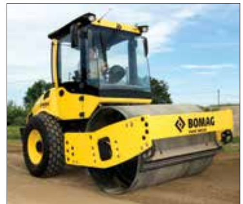
Models are suitable for compaction of granular, mixed and semi-cohesive soils.
