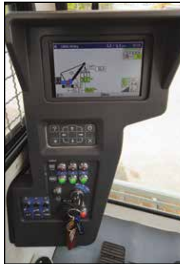
HSL capacity limiter with high visibility color graphic display
