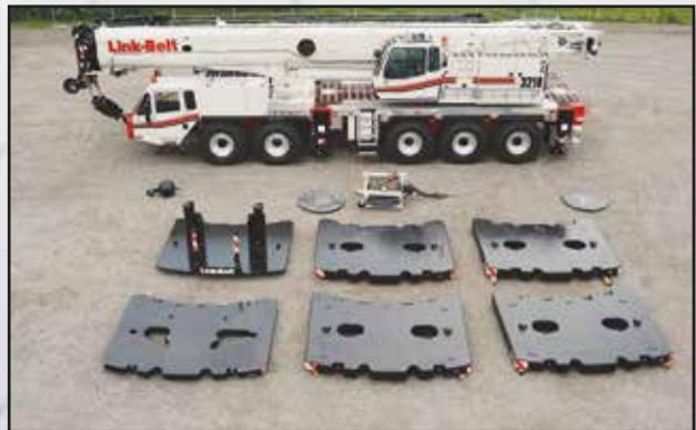
↑ Auxiliary winch can be removed and installed without an assist crane using only the bottom tray of the counter weight stack. A newly designed counterweight removal system allows all counterweight configurations to be raised and lowered by hydraulic cylinders from the comfort of the operator's cab.
