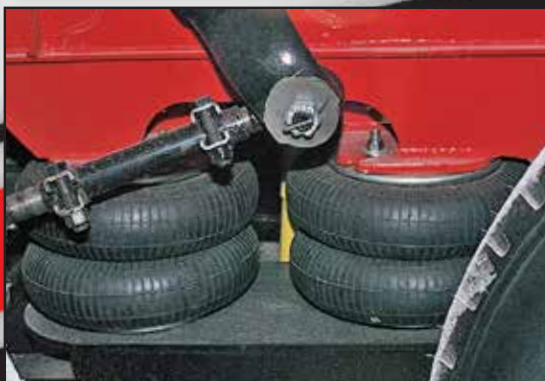
Air-ride suspension front and rear provides a smooth ride and precise handling. Optional air-ride lift system holds the rear suspension retracted while the crane is on outriggers.
