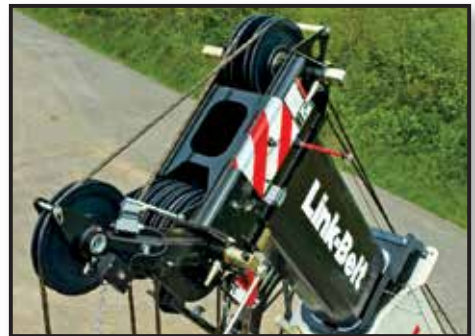
Quick reeve boom head eliminates the need to remove the bucket when it becomes necessary to change the reeving.
