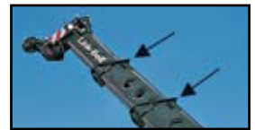
A-max extends only the inner-mid section of the boom for substantially increased capacities for in-close, maximum capacity lifts.
