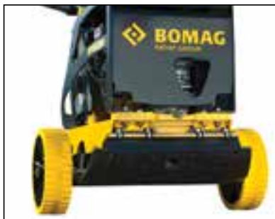
The transport wheels allow for one-person movement around the jobsite.
