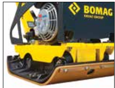
The Vulcolan mat helps avoid damage to paving stone surfaces.
