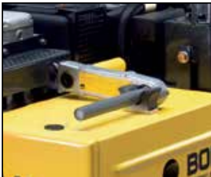
Standard electric start with back-up crank handle.
