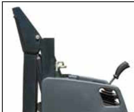
The standard foldable ROPS offers flexibility for transport and storage.
