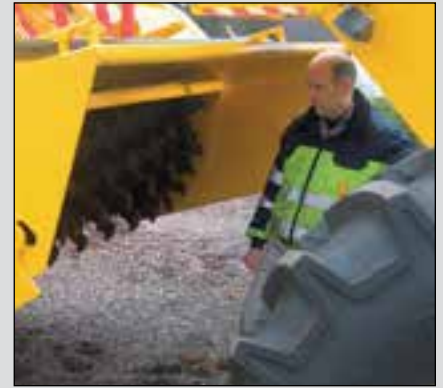
Quick replacement of cutting teeth without the need for special tools.
