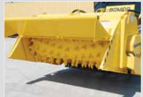
Easy and convenient replacement of cutting teeth without special tools.
