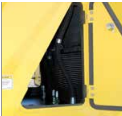
Wide opening hoods and access doors provide easy access to maintenance items and for cleaning purposes.
