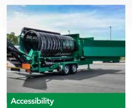
The screen drum is freely accessible by opening the large side door. To change segments, the drive chain is loosened and the drum lifted out of the machine with suitable lifting gear. With the "Drum Grip" system there are no teeth welded on the drum
