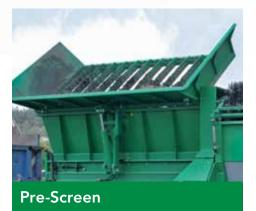
When working with excavated material, aggregate or lightweight building debris, a grizzly prevents damage from large overs. The sturdy coarse material grid folds hydraulically by remote control and has a chute to eject overs beside the machine.
