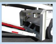
Hydraulic conveyor lift on Discharge conveyor.
