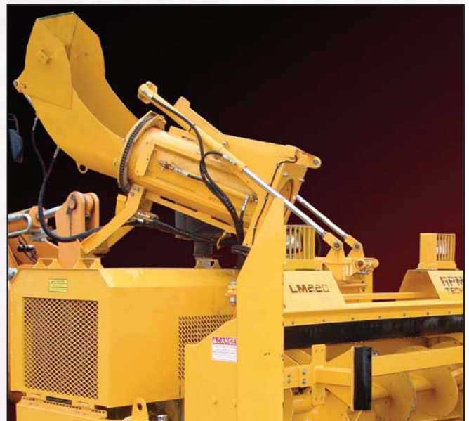
Optional hydraulic tilting chute: • Better visibility when traveling; • Easy cleaning of the chute when clogged with snow.
