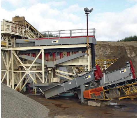
Designed to remove large volumes of excess water from feed material, the Eagle Water Scalping-Classifying Tank is typically used in such applications as dredging and pumping and with high silt materials. It smooths out feed fluctuations and is key to removing excess sand particles for a consistent, reliable in-spec product.
