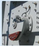
Heavy duty bearing housing with remote lube and adjustable counter-weight.
