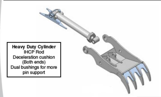
All PSM Thumbs can be custom engineered and manufactured to fit properly with your existing buckets and quick couplers, at no additional charge. 100% T-1 Construction CNC Machined Dual heat treated pins Hardened bushings
