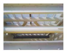
ensures high structural strength and rigidity. Access to the decks is easy through our swing-down back plates. Crown bars are contoured and stitch-welded to the cross beams, rather than just welded to the tops of the beams.
