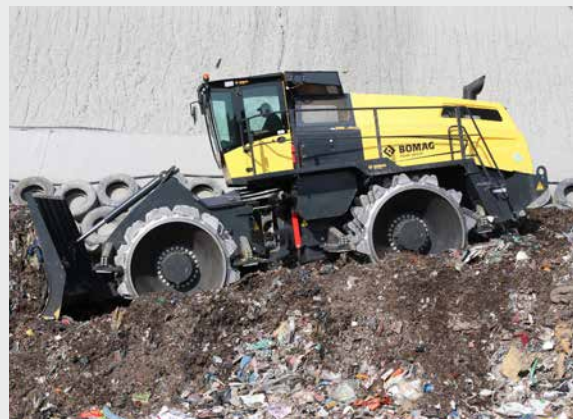
Optimum compaction with the oscillating joint, providing good load distribution to the compaction wheels.
