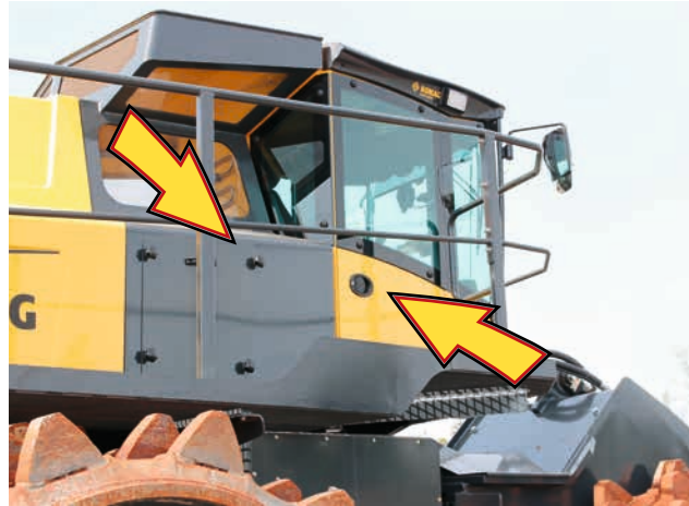
Access to the radiator and maintenance opening for the air conditioning unit.
