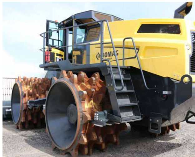
The service platform provides access to the maintenance area.
