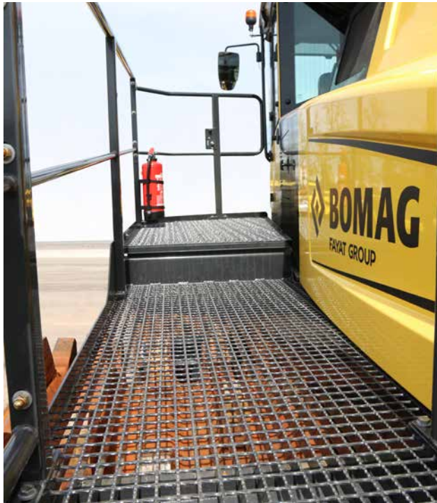
Open stairs and the platform structure keep things clean.
