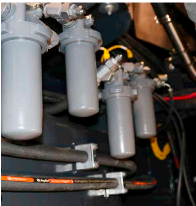
Hydraulic filter system.
