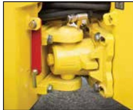
Maintenance free bolt on articulated / oscillating joint.
