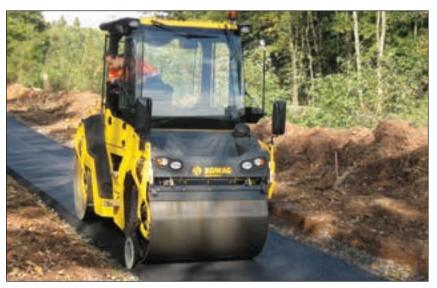
The optional cab and edge roller features will increase machine versatility for all weather conditions
