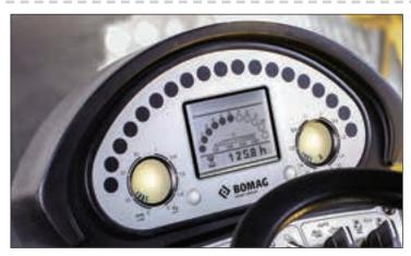
The optional ECONOMIZER indicates compaction results. Simple and easy, to save time, prevents unnecessary passes, and avoids over-compaction.
