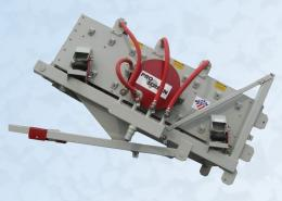
4 Bar Wash System with 7 spray nozzles per bar, 1 1/2" brass gate valves, water manifold with 3" inlet, and clean-up hose hook-up. (Requires 140 gpm at 40 psi water source)
