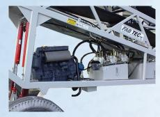
Deutz F4L2011 air cooled diesel has 55 hp at 2100 rpm
