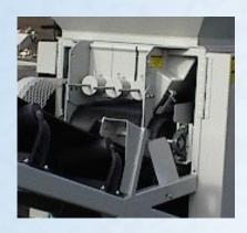
24"x5' belt feeder hopper has adjustable weighted feed gate.
