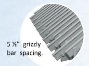
Separating grid grizzly is easily cleared by lifting the grizzly which allows rocks to dislodge.
