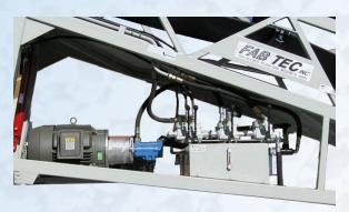
40 HP TEFC motor ~vs~ Deutz diesel to run the hydraulic pump.
