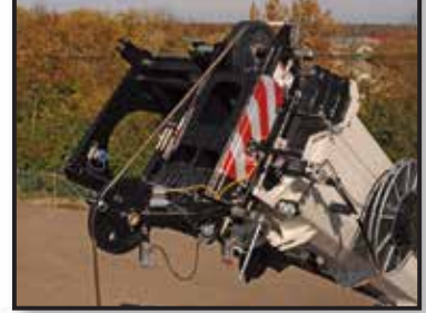
Quick reeve boom head eliminates the need to remove the becket when reeving is changed.
