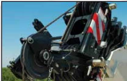
Quick reeve boom head eliminates the need to remove the bucket when it becomes necessary to change the reeving
